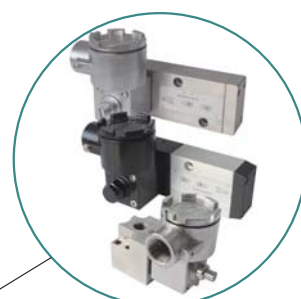
Solenoid Valve 3/2NC & 5/2 Way, Static O-ring Sealing Design. Aluminum & 316SS Body IP67 & EExdIIBT6/EEExdIICT6
